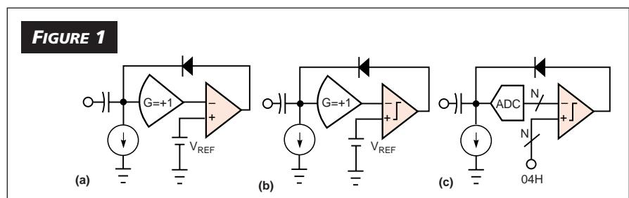
Sync-tip clamping using either an op amp (a) or a comparator (b) is a common technique for sync detection. Digital sync-tip clamping (c) embeds an ac-coupled ADC in the clamping feedback loop, a scheme that performs dc restoration without horizontal-timing information.
